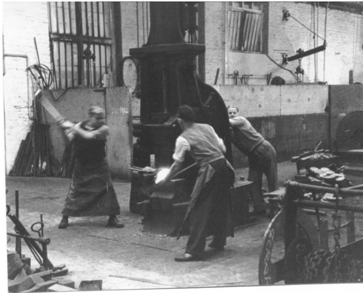
Blacksmiths, Swindon Railway Works. Blacksmith Ted Mitchener working a hot billet with a sledgehammer. Striker Charlie White uses tongs to assist while the piece is held firmly under the steam hammer with Reg Terry the hammer driver at the controls.
